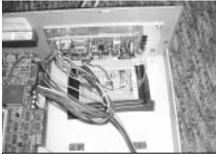
Completed power supply and delay circuit installed in my 386 computer.
